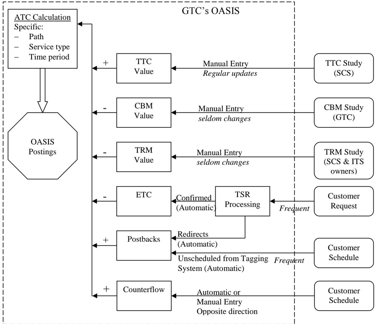
This process flow diagram illustrates the various steps through which a single ATC (based upon specific factors) is calculated. Similar ATC calculations are performed for each path, service type, and time period and will generally result in different ATC values specific to those factors.
